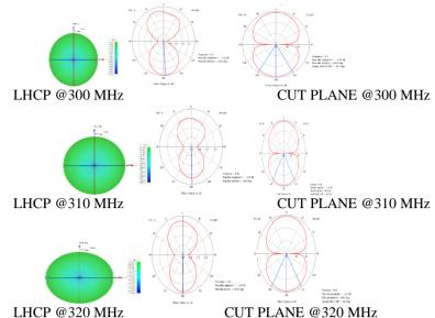
**Fig. 5.** Radiation patterns of UHF Crossed dipole antenna at various operating frequencies.
